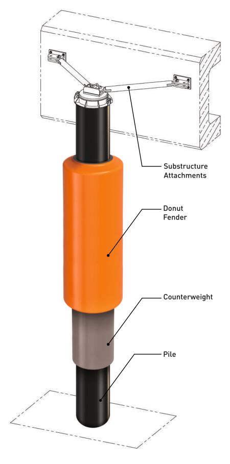
Hi-Tech Donut Fenders are also designed to provide a high rate of energy absorption with a relatively low reaction force. It is designed to simply slip over a stationary monopile and float at the fluctuating water line.
