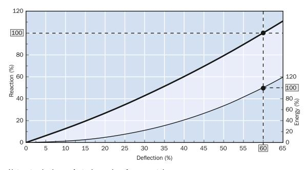
Note: standard manufacturing and performance tolerance: Energy: 100%, reaction: 100%, Tolerance: ± 10%
