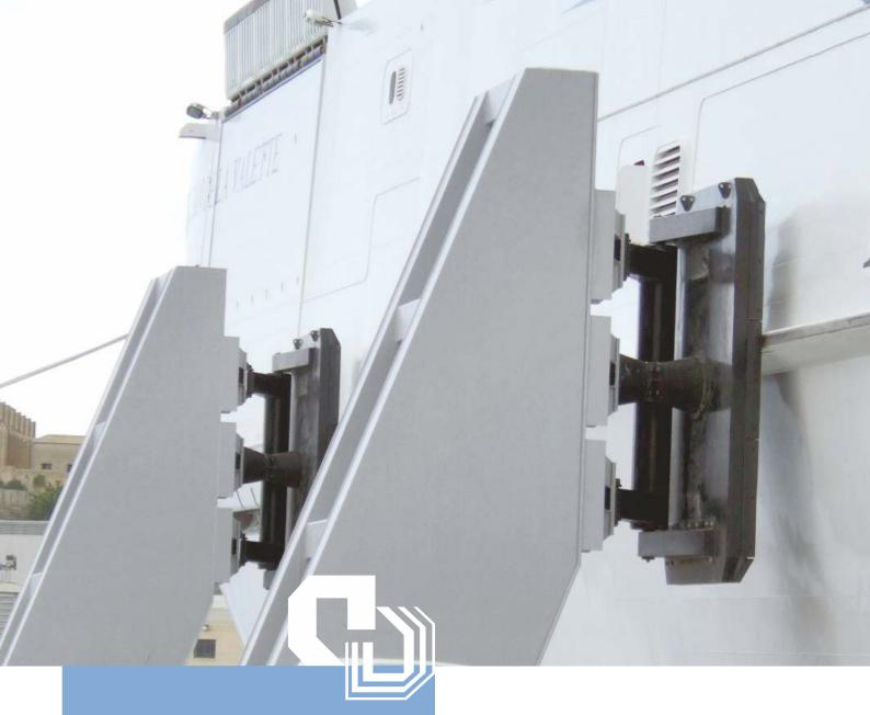
Parallel Motion technology can reduce reaction forces by up to 60% compared with traditional designs.
